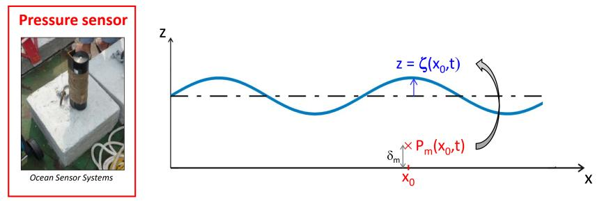
**long waves**: tsunamis, tides, ... → **<u>hydrostatic reconstruction</u>**
