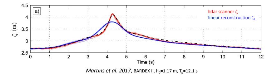
$\rightarrow$  provides a poor description of the peaky and skewed shape of nonlinear waves  $\rightarrow$  underestimates the individual wave height by up to 30 %
